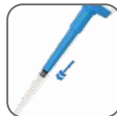
Eject Tips Easily with a Tip Ejector
