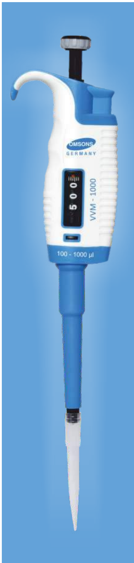
Adjust Volume Easily with Plunger
