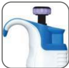
Adjust Volume Easily with Plunger
