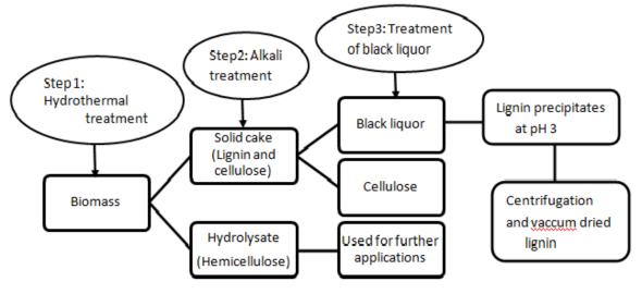
Fig 1: The schematic description Extraction and isolation of lignin from biomass (herbivorous animal manure)
