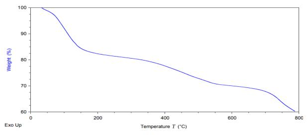
Fig. 4: TGA thermograms of lignin
