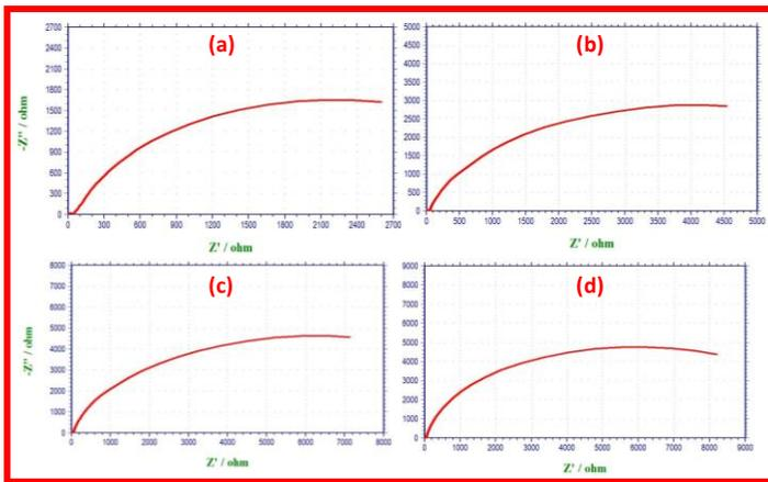
Fig. 2. Nyquist plots of (a) As cast (b) 2% Al<sub>2</sub>O<sub>3</sub>+9% SiC+180 °C aging temperature, (c) 4% Al<sub>2</sub>O<sub>3</sub>+9% SiC+180 °C aging temperature, (d) 6% Al<sub>2</sub>O<sub>3</sub>+9% SiC+180 °C aging temperature.
