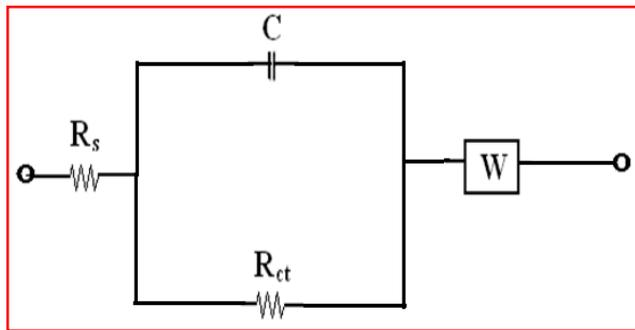
Fig. 3. Proposed equivalent circuit of Nyquist plot.
