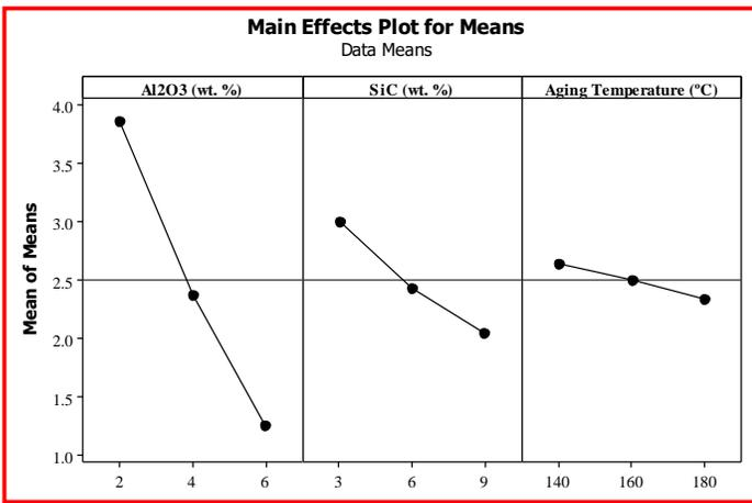
Fig. 4. Main effects graph for corrosion loss
