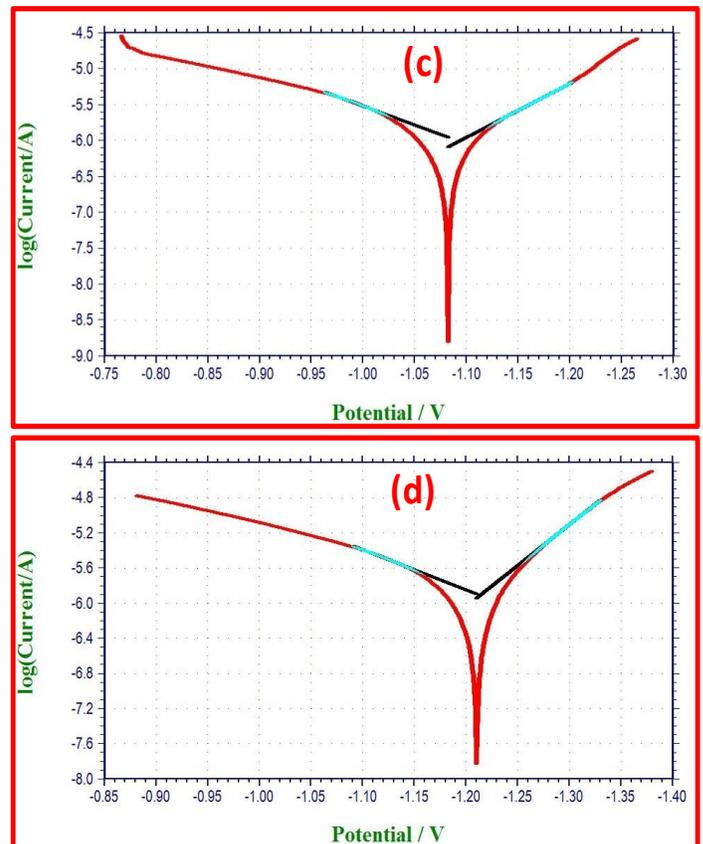
Fig. 1. Polarization curves of (a) As cast (b) 2% Al<sub>2</sub>O<sub>3</sub>+9% SiC+180 °C aging temperature, (c) 4% Al<sub>2</sub>O<sub>3</sub>+9% SiC+180 °C aging temperature, (d) 6% Al<sub>2</sub>O<sub>3</sub>+9% SiC+180 °C aging temperature.
