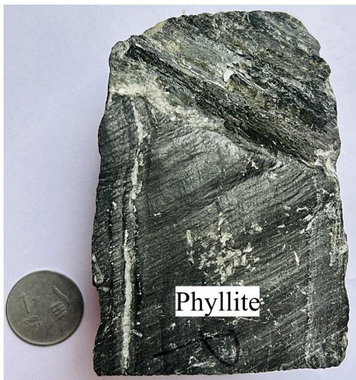
Fig. 2. Hand specimen of carbonaceous phyllite, host rock of Mochia-Magra Pb-Zn Mines. The silky and satiny sheen luster with strong fissility is a diagnostic feature of phyllite, a low- to medium-grade metamorphic rock. The rock exhibits parallel alignment of very fine-grained platy minerals with shiny surface.
